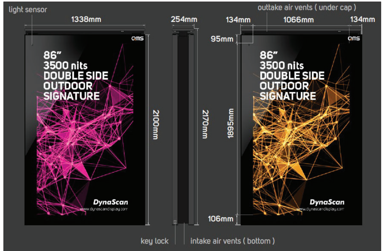
Digital Signage Panel Dimensions. NTS (Source: Dynascan)
